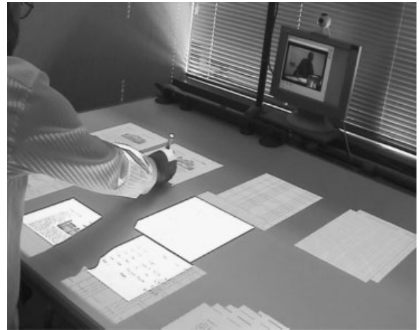
Figure 2. We have linked two Escritoire desks to create a large shared visual space between participants containing document and images. They can also see and hear each other via a conventional videoconference.
