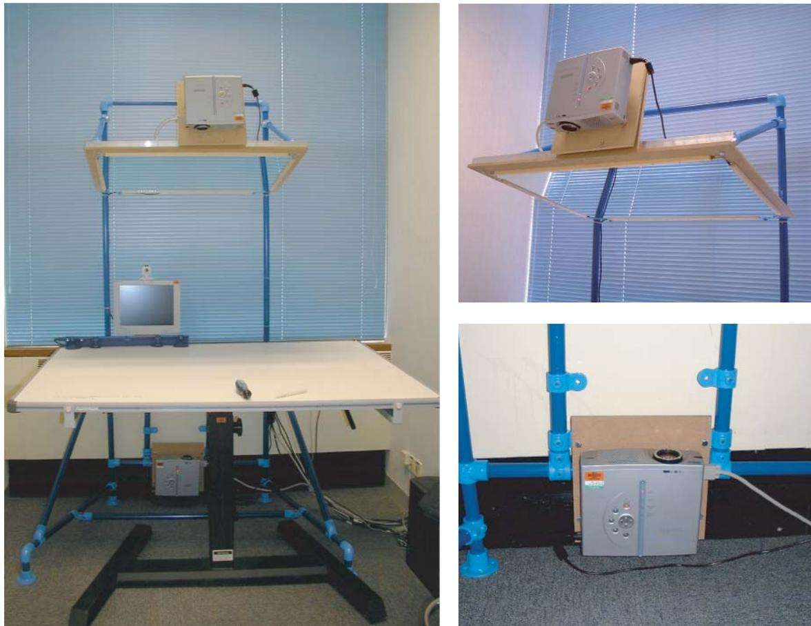
**Figure 3.8:** The second version of the Escrtoire hardware. A purpose-built frame (left) holds the two projectors and the large mirror. The top projector is mounted at a steep angle (top right) so there is no need for a mirror to reflect it's image downwards. The bottom projector (bottom right) points upwards, towards the large mirror.
