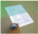
Pens in both hands are used to arrange and manipulate the items on the desk. A stateless, hardware-dependent client program handles the desk, while a separate server manages the desk contents. Multiple clients augment the 'person space' of a conventional video conference with a 'task space' that the participants share.
