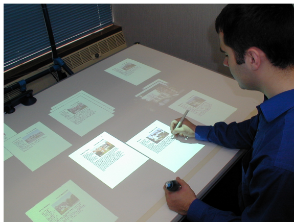
Figure 5: The Escritoire is a large horizontal display and interaction device that provides much more space than a normal computer monitor, and interaction that is more like using physical papers on a traditional desk.
